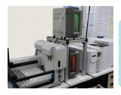
Instruments such as purge and trap gas chromatography-mass spectrometer (**P&T GC-MS**) or a liquid chromatography-mass spectrometer (**LC-MS**) in the lab
