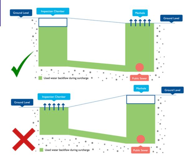
The floor level of the development and the levels of the sanitary appliances, floor traps and inspection chambers should be constructed at levels higher than the manhole to which it is connect to.
