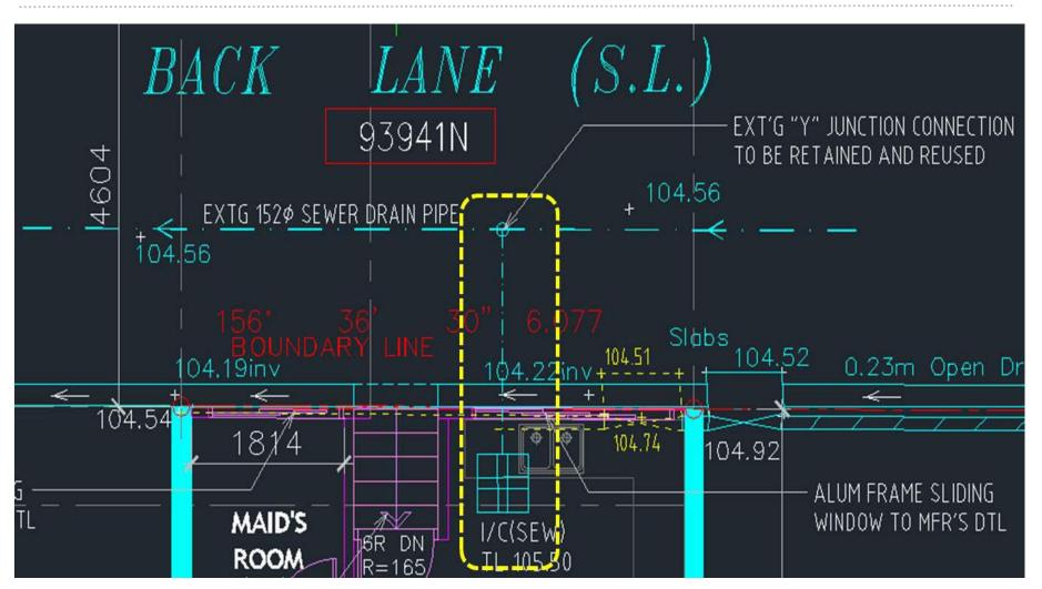
The point of sewer connection that serve the development must be shown clearly.
