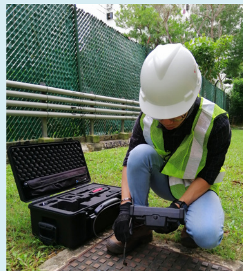
▲ Manhole Inspection via Keyhole Deployment
