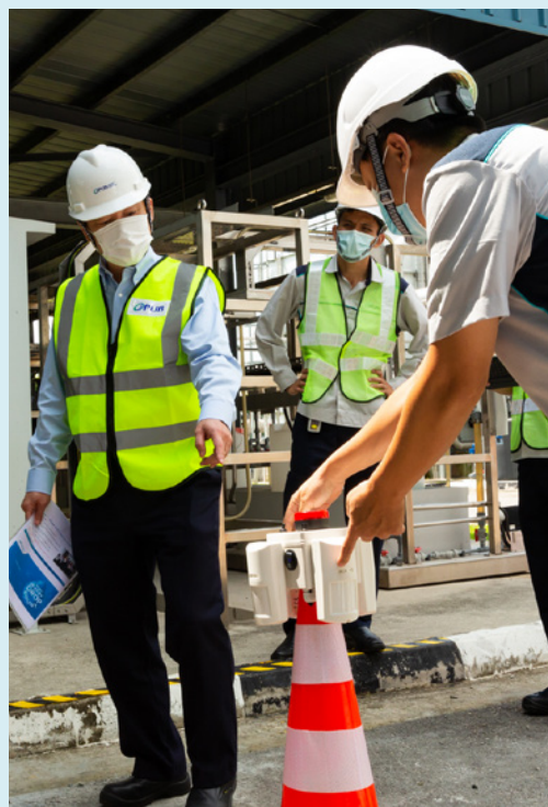
▲ Screaming Cone – Sensor Activated Alarm System
