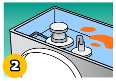
Sprinkle food colouring (or drop a leak detection tablet) into the flushing cistern tank, and observe the toilet bowl for any coloured water. Did you know a leaking flushing cistern tank can lose more than 10 litres of water per hour?
