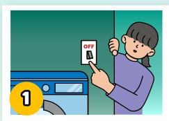
Turn off all taps and appliances using water, and monitor your water meter for at least 10 minutes. If the meter dial moves, there is a leak.
