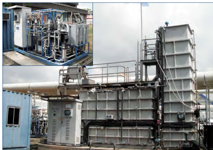
Fig. 2: Toray's pilot plant couples the double-decked Membrane Bioreactor (MBR) to a Reverse Osmosis (RO) process
