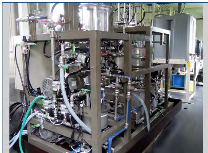
Fig. 2: Non-chemical Feed Filtration System used to test the removal of fluoride
