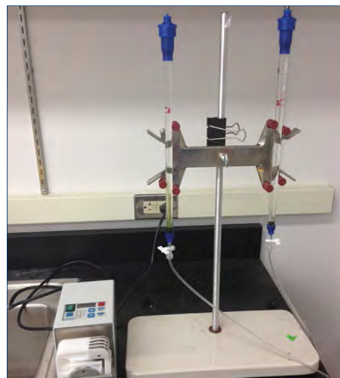
Fig. 2: A bench-scale GAC column used in the study
