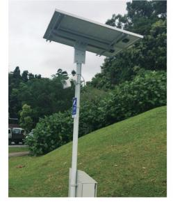
Figure 1. CCTVs are designed to record and monitor scenes. However, by harnessing advanced technologies, they can be also be used as a rain gauge.
