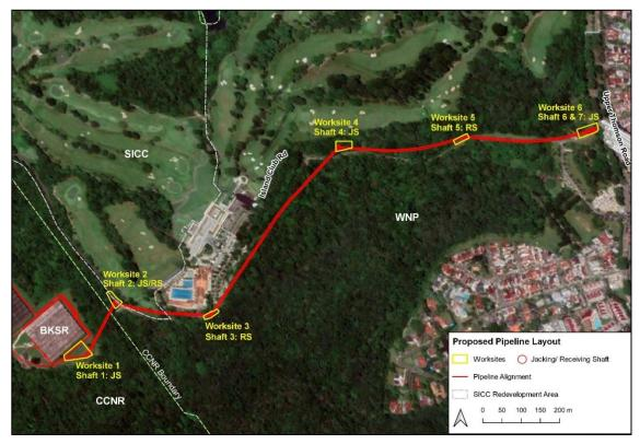
Figure 3: Layout Plan of the Shafts and Pipeline
