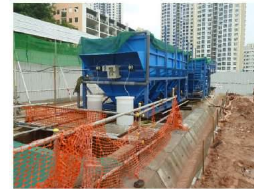
Chemical ECM Silt Treatment Plant flow rate from 5m 3 /hr. to 80m 3 /hr. c/w with submersible pumps and auto discharged valve for certain models
