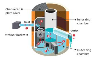
Without the grease trap, grease will enter the sewers and accumulate, resulting in encrustation. The encrusted grease may obstruct the smooth flow of used water in the sewer and cause it to overflow into your premise or other public areas.
