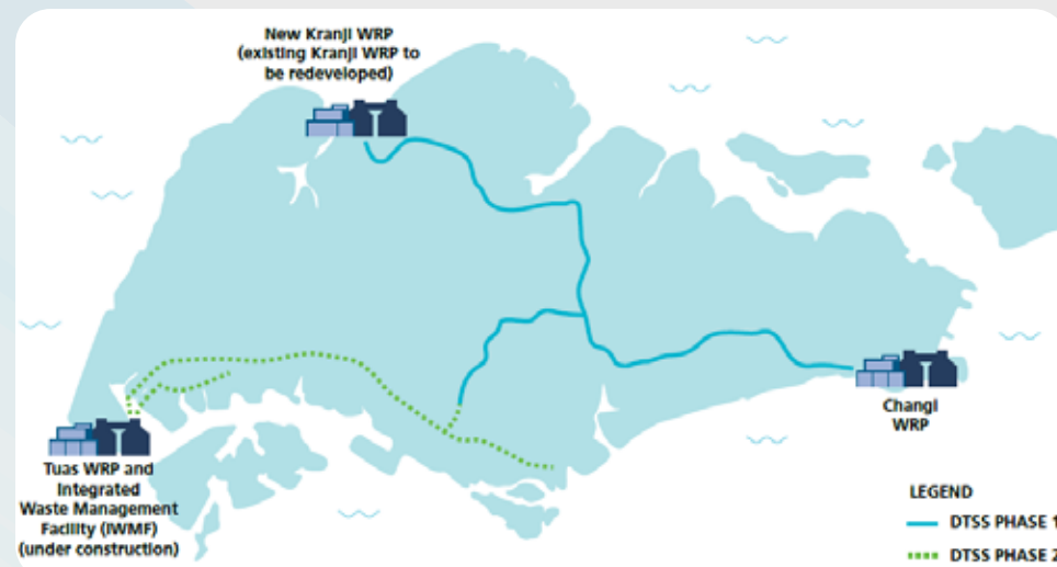
Singapore's three-node used water system.
