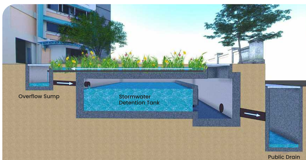
Figure 1.10 Acting as a source measure, the construction of a detention tank below a rain garden, helps to retain the first flush stormwater runoff while simultaneously cleansing it. Any excess runoff will overflow into the detention tank.
