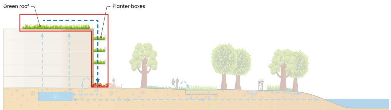
Figure 3.12 On-site stormwater detention and retention options on buildings.
