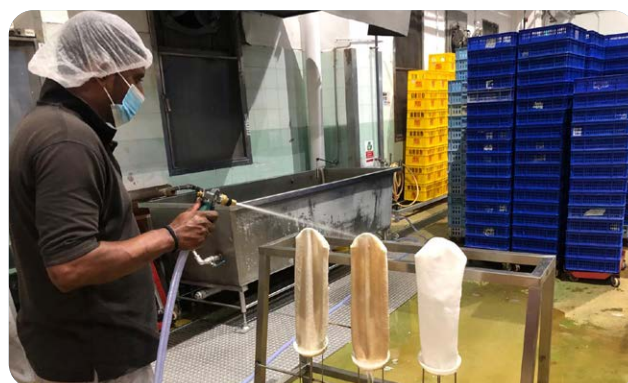
A VIS employee washes the filter bags that help to remove large impurities from overflow water.
