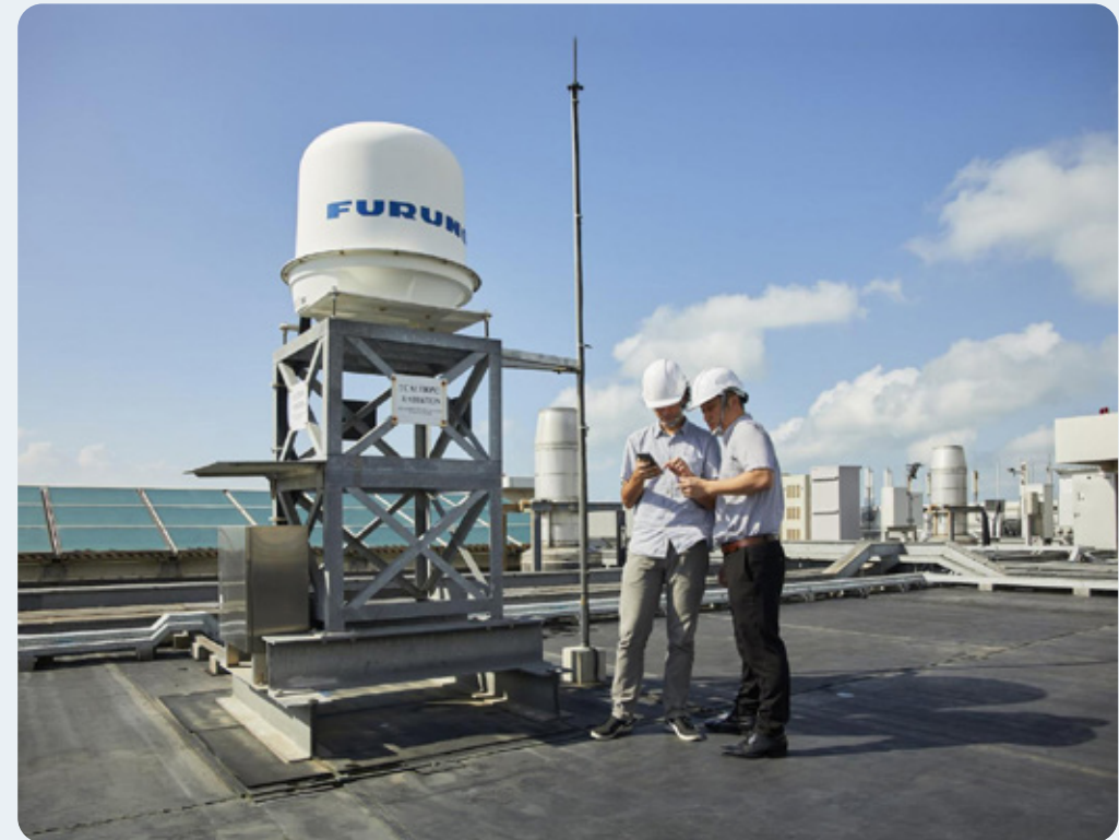
An X-band radar, developed with the Hydroinformatics Institute and Furuno Singapore, placed on top of a building rooftop.
