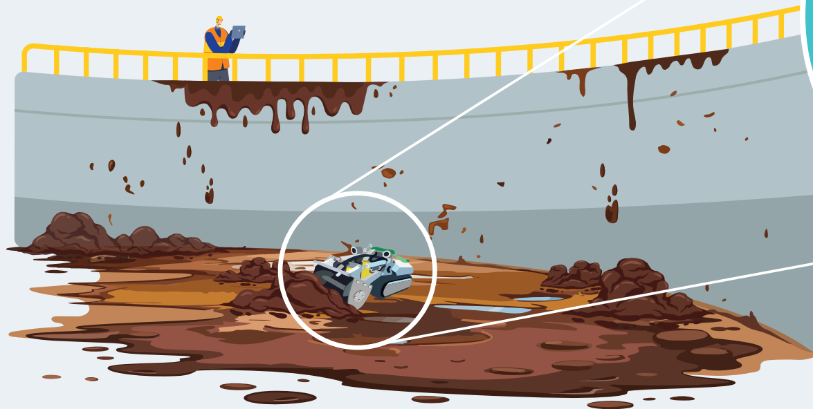
Remote-operated robotic cleaner for confined space cleaning.
