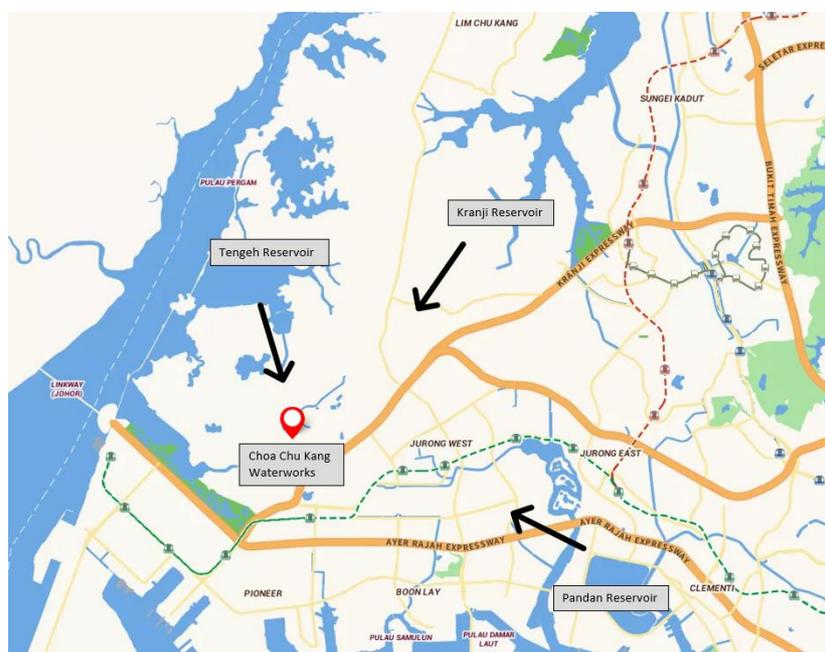
*Figure 1: Location of CCKWW and surrounding reservoirs. Arrows indicate direction of water flow from the reservoirs to CCKWW.*
