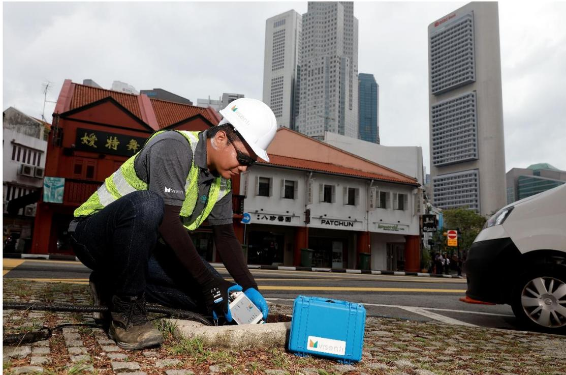
*Real-time pipe failure detection. Visenti's LeakView™ system is comprised of multiple pipe leakage indicators such as high-rate (64-256 samples/sec) pressure sensors, hydrophones and flow meters installed at optimal locations - coupled with minute-by-minute data analytics for anomaly detection.*
