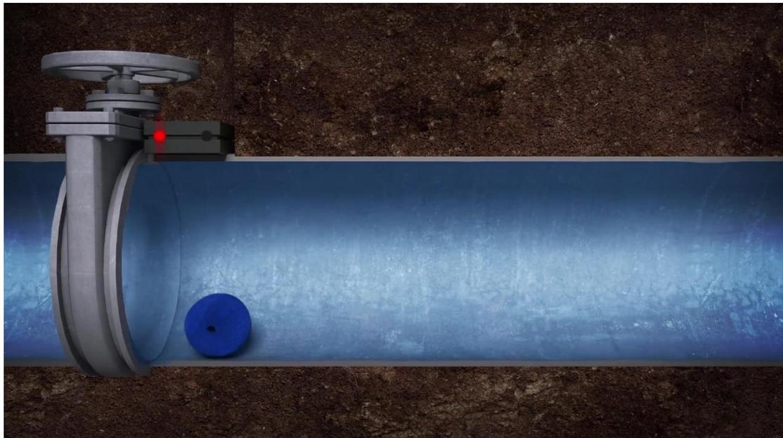
*Pure Technologies' SmartBall is a key solution in reducing water loss in previously neglected assets by detecting leaks on large diameter mains, helping utilities locate and repair leaks before they surface. The SmartBall tool is inserted into a pipeline and travels with the water flow for up to twelve hours while collecting information about leaks. It requires only two access points for insertion and extraction, and is tracked throughout the inspection at predetermined fixed locations.*
