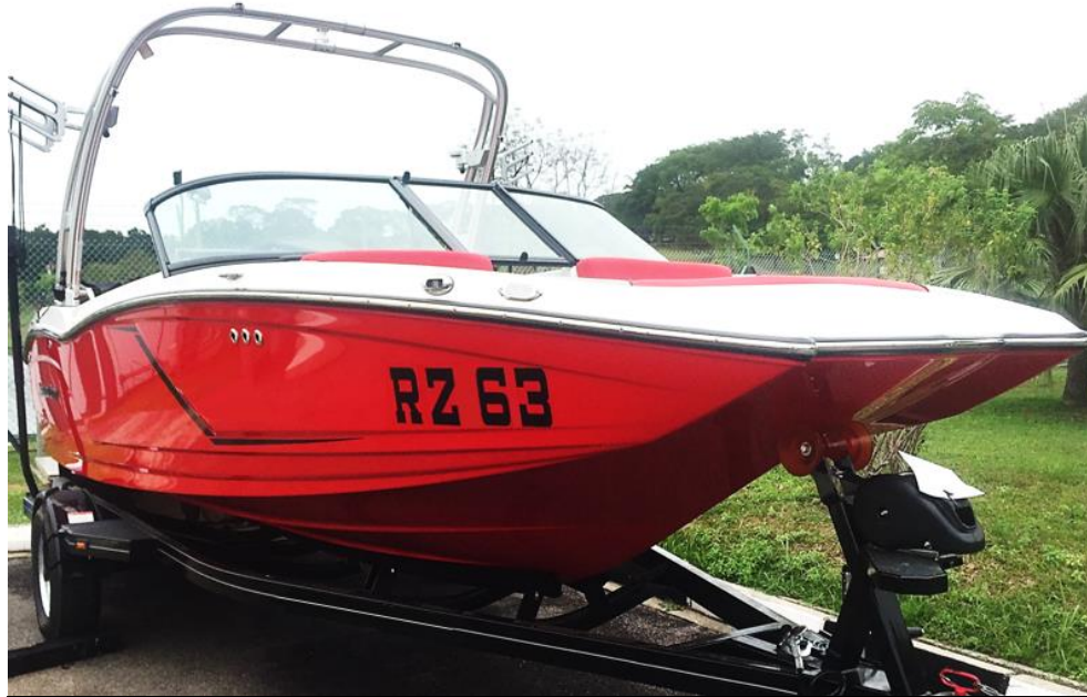
Vessel ID (not lesser than 150 mm in height) prominently painted on both sides of the vessel
