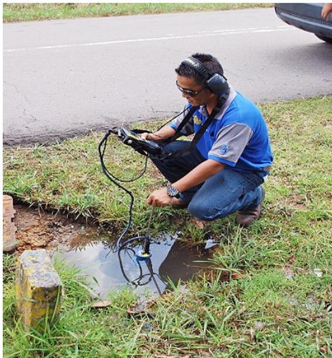
*Staff using a ground microphone to verify and pin-point leak location.*
