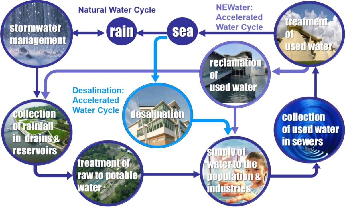
The Concept of a Closed Water Loop
