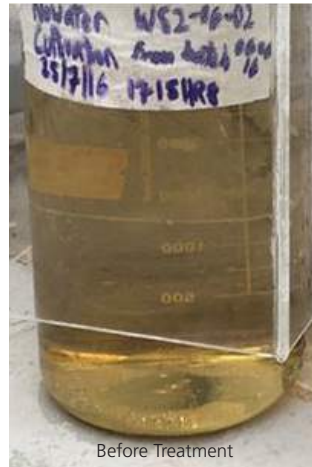
Fig. 2: NF hollow fibre membranes were used in a laboratory-scale treatment of reverse osmosis retentate in NEWater production. The results showed a clear difference in colour between the untreated and treated samples
