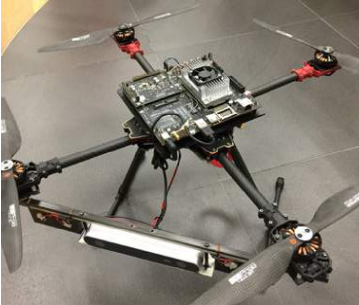
Fig. 1: A miniature unmanned aerial vehicle (UAV) for use in inspecting the Deep Tunnel Sewerage System
