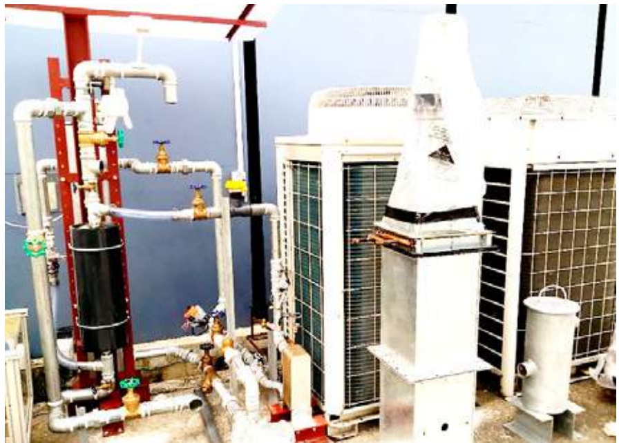
Fig. 1: The laboratory prototype of the membrane-based evaporative cooler (MEC) system (left), compared to a conventional cooling tower (right)
