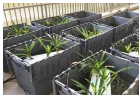
Fig. 2: Aquatic plants being tested for their ability to take up nutrients in water
