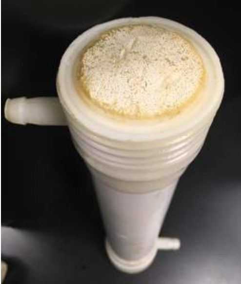
Fig. 1: The cross-section of a 1-inch nanofiltration (NF) hollow fibre module
