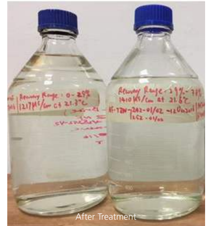
Fig. 2: NF hollow fibre membranes were used in a laboratory-scale treatment of reverse osmosis retentate in NEWater production. The results showed a clear difference in colour between the untreated and treated samples
