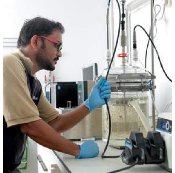
Fig. 2: A laboratory analysis of the biogas methane potential of the sludge produced
